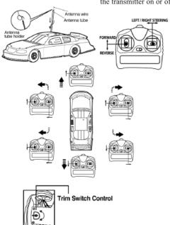
Trim switch is located on the underside of the vehicle, between the two front wheels, and is used to align the wheels for consistent straight line driving.
